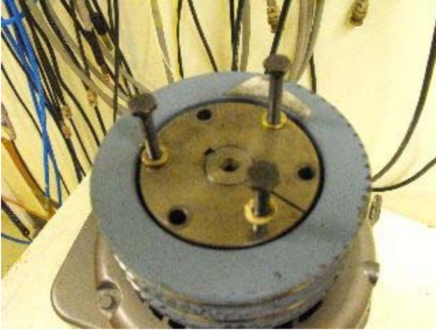
Relocate the bolts to the threaded holes in the bushing.
