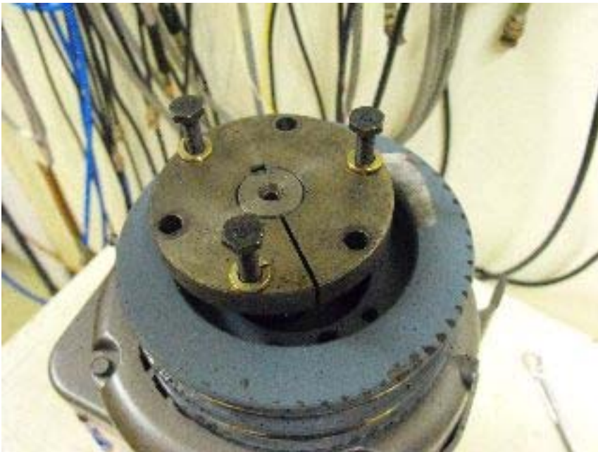
Tighten bolts evenly and the sheave will drop away from the bushing.
