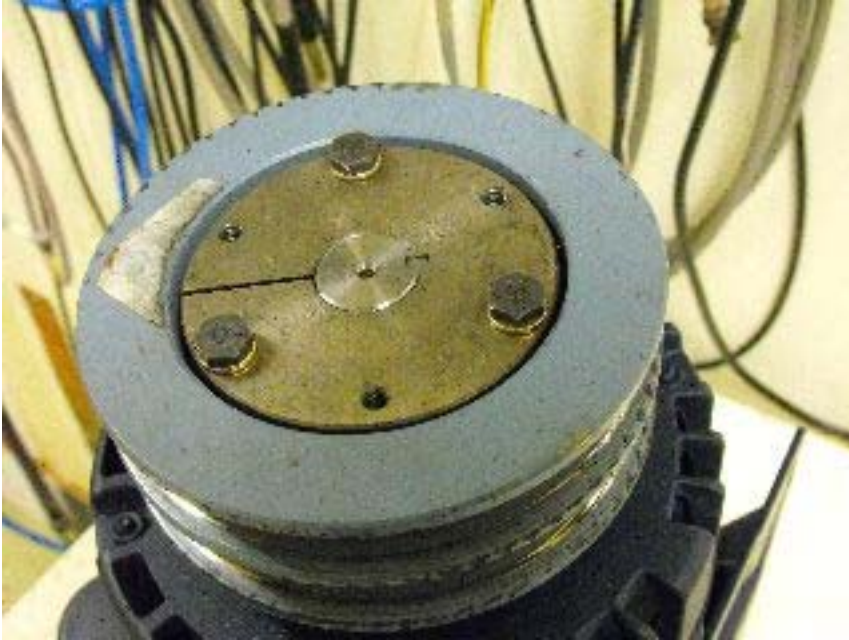
Tighten bolts, alternating between bolts to ensure sheave slides evenly onto bushing.
