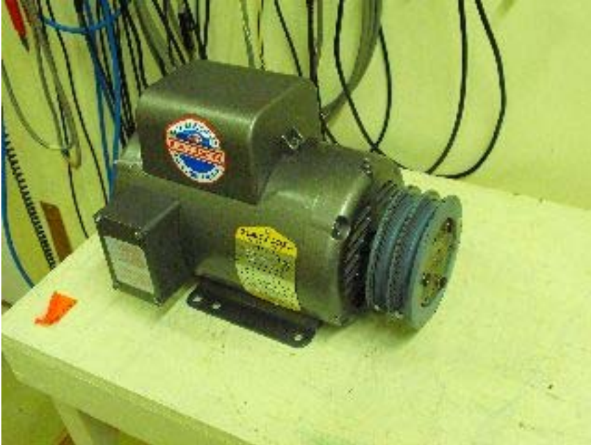
Original motor. Bearings damaged and making loud growling noises while motor is running. Take note of the pulley position on the shaft such that it can be installed in the same position on the new motor.
