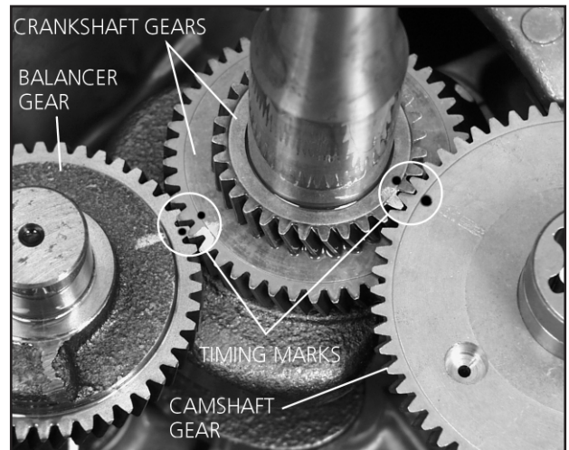
Figure 11.11 — Alignment of Timing Marks
