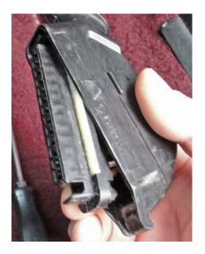
Lever the terminal assembly out of its case. (Rear section fits under a tab.)
