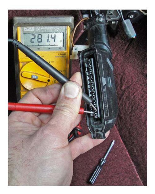
Check resistance between terminals 12 and 25 as shown with throttle depressed fully, or a jumper inserted between B and C at the engine test port.
