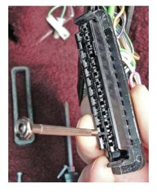
Push in to release terminal catch (#12) as shown. WOT input is two wires, white with red stripe.
