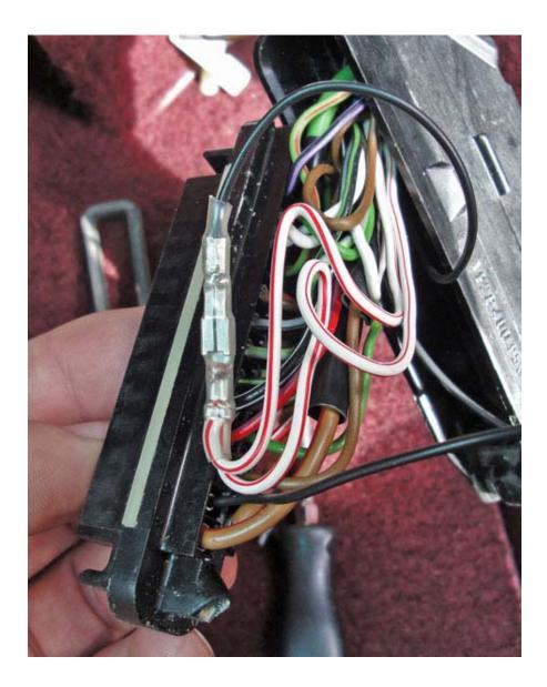
Feed WOTpot wires into rear of case.
