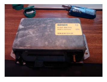
Starting with the EZF, there are tabs around the perimeter of the case that must be pried up. EZF is the computer with the vacuum port. After removing the case, the circuit board will be exposed (attached to the flat part of the case.)
