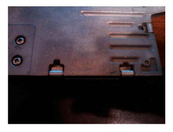
These tabs must also be pried up to allow the cover to come off. Being recessed, they can be a little tricky, but on mine, all but one came up easily with a screwdriver slid through the notch and underneath the tab. The last one I used a jeweler's screwdriver on the upper part of the tab. Be careful not to break them.
