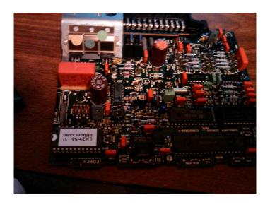
The new LH2'r installed. Again, pay attention to the orientation of the notch on the chip and make sure it matches the notch on the socket. In this case, you'll need to separate the LH2'r from the shipping socket, as the board will not seat with the extra height. It's very easy to accidentally bend the pins when removing the shipping socket, so be careful.
