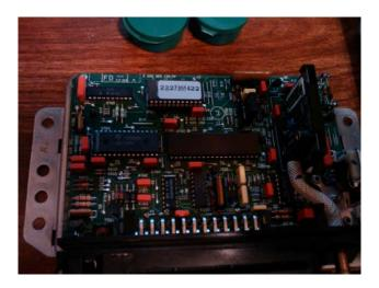
At the top of the picture, the stock chip sits in a socket. Apply gentle pressure underneath with a small screwdriver. Take care not to touch the pins if you can help it. Also, try to remove the chip evenly to avoid bending the pins. It's not unusual to bend one of the corners as you remove it. Notice the notch in the chip and the notch on the socket as well.
