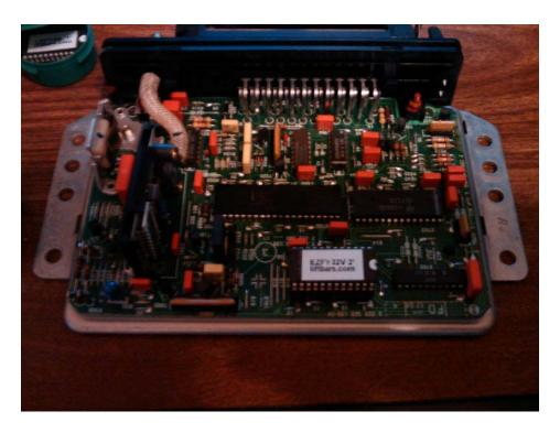
Install the new chip with the dotted side (in this case, marked clearly in white) on the notched side of the chip holder. The socket that comes on the chip is probably intended to make sure the pins don't get bent. You can install the EZF chip with or without, it shouldn't matter much. Reassemble the case and bend the tabs back around to make a firm fit.
