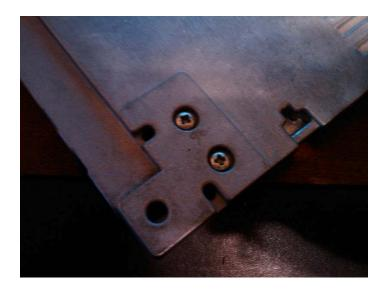
These screws must come out as well, they're attaching some transistors to the big metal plate for cooling purposes. Also, the Philips screw that holds the plug retainer must be removed to allow access to a second Philips screw beneath it. Pay attention to the plug retainer clip orientation, although if you forget which way it goes, it installs in the way that makes it inconvenient to get the second screw out.
