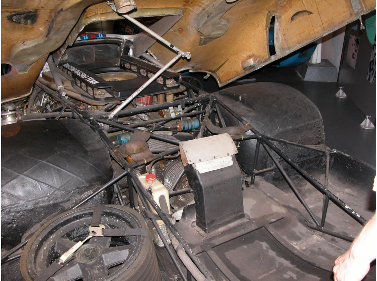
12 CYLINDER ENGINE OF PORSCHE 917 LH No. 21: 1971 MARTINI RACING TEAM
