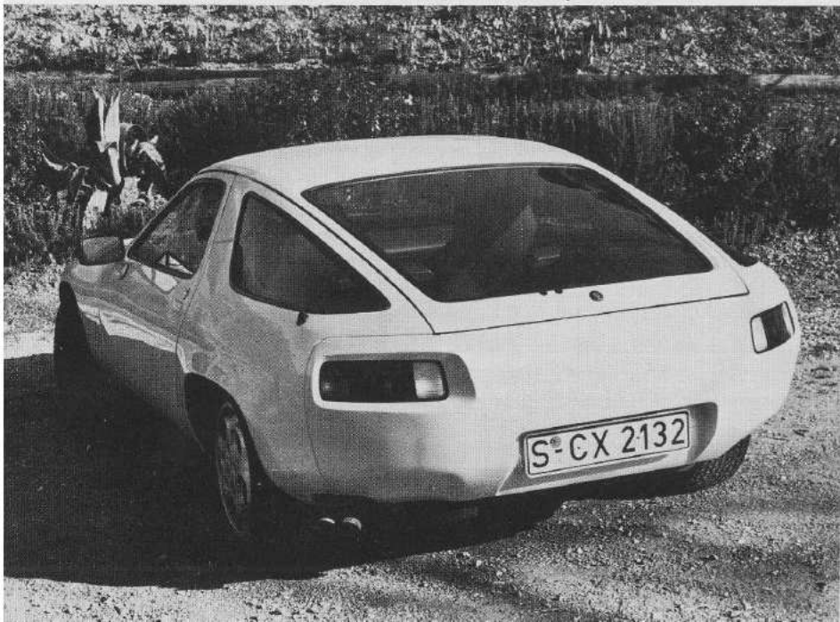
Good integration of polyurethane bumpers with body was achieved in 928 design.
